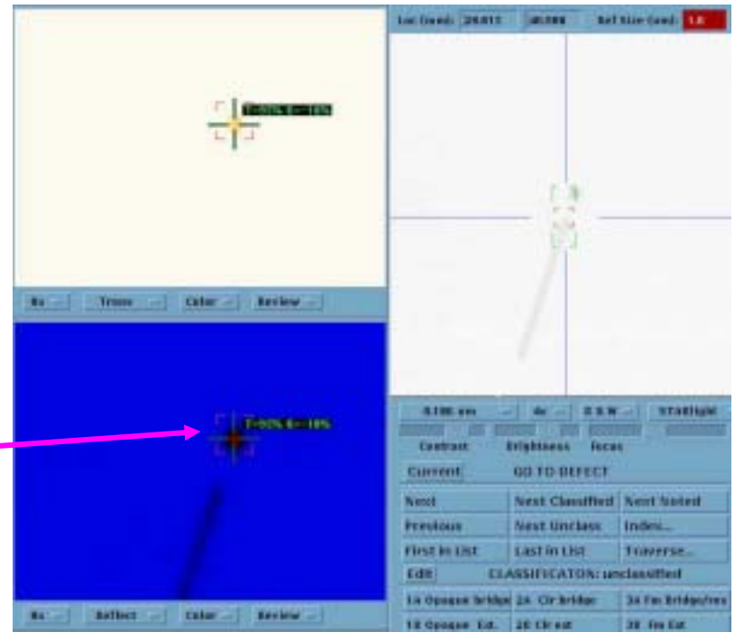
A very narrow comet defect with 5% transmission loss
